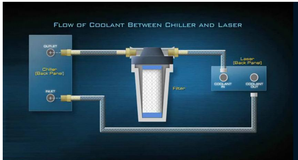
Figure 4-1 Water Hoses and Filter Connections
